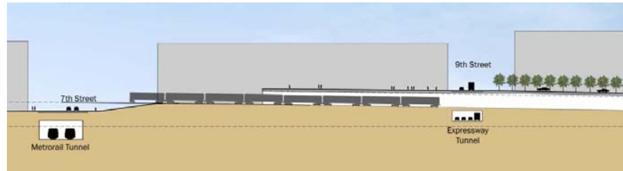
Section along the centerline of Maryland Avenue SW illustrating the proposed decking over the railroad - view to the southeast
