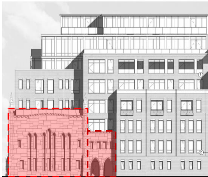
Incompatibility of proposed addition's scale to the existing 1922 Parish Hall (in red).
