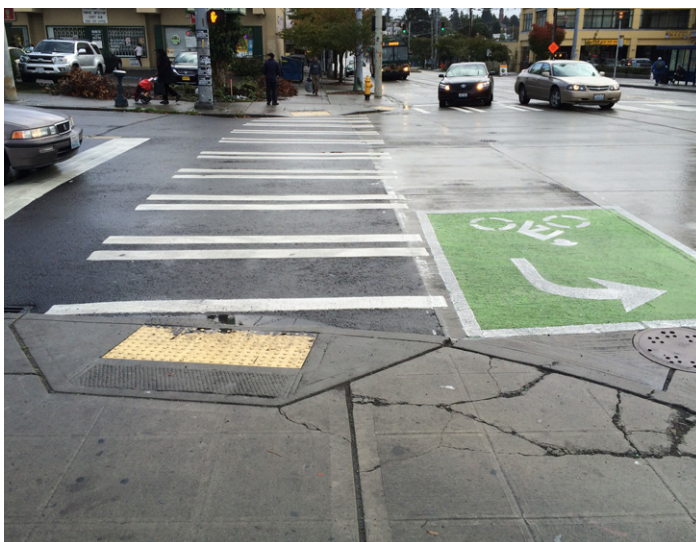
Two-Stage Left Bicycle Turn Queue Box
