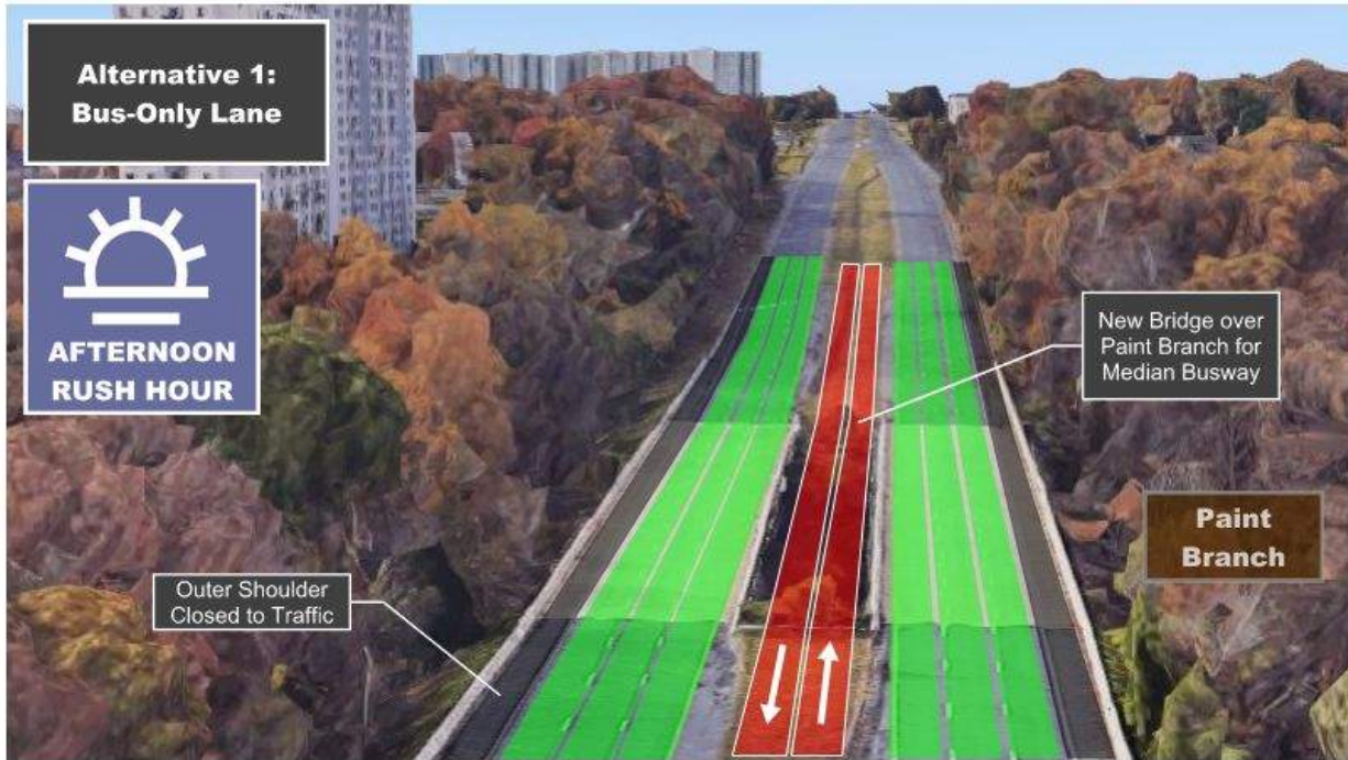
Figure 5. Median Bus Lane Alternative at Paint Branch
